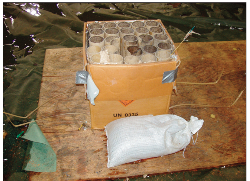
A "finale box" of 25 mortars designed to be lit once.
